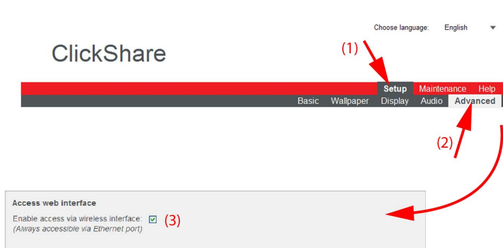
Image 6-26 Access web interface
